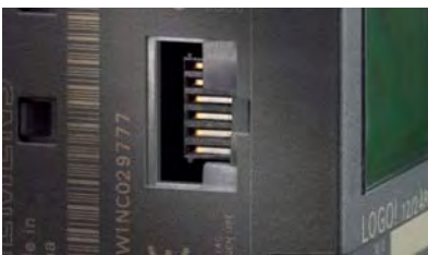
Simple connection of the LOGO! TD text display
